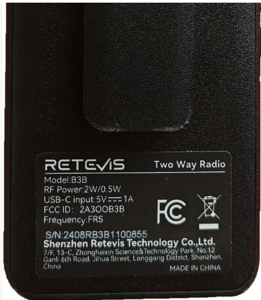
Figure 8: Back of Retevis B3B with specifications.
