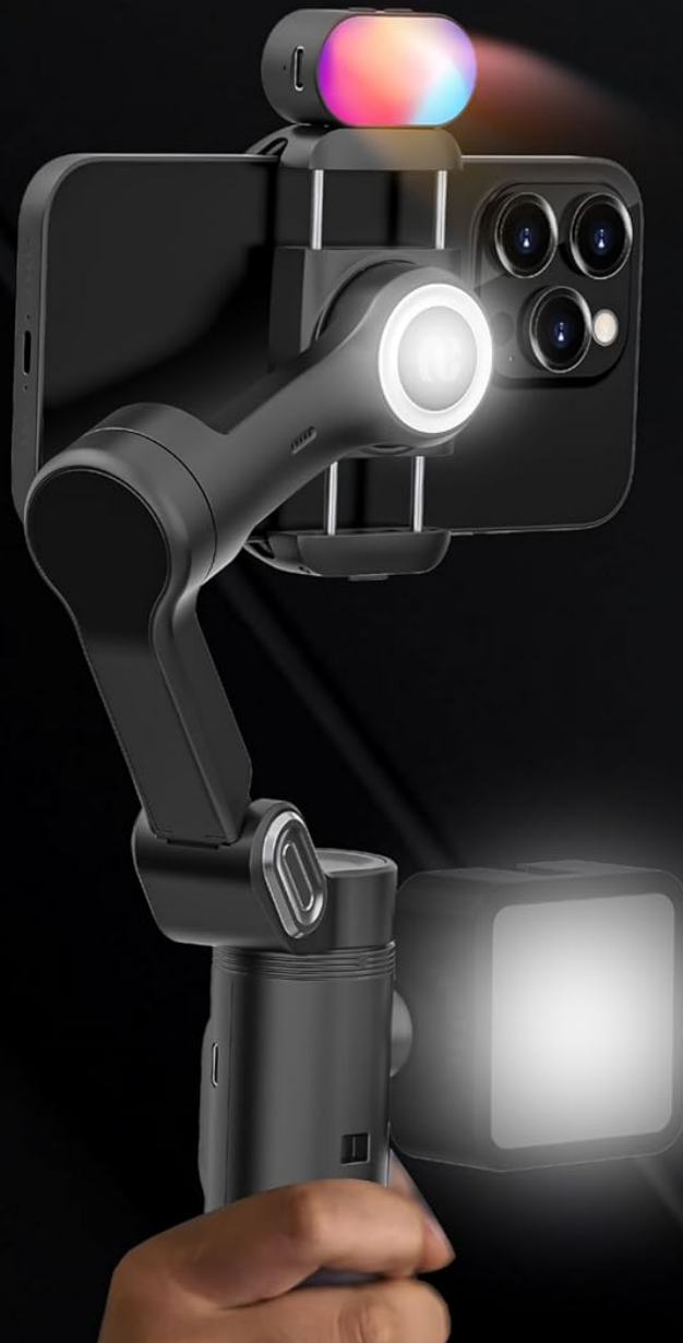
Image 6: The gimbal's built-in ring light and magnetic RGB light providing illumination.
