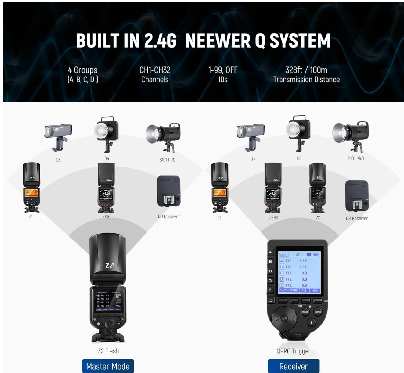
Image 5.1: Overview of the NEEWER 2.4G Wireless Q System, showing groups, channels, and IDs.
