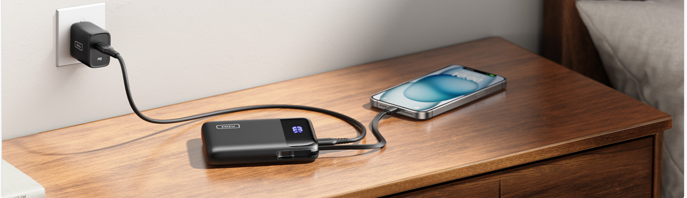
Figure 8: Illustration of pass-through charging, where the power bank is recharged from a wall outlet while simultaneously charging a connected smartphone.
