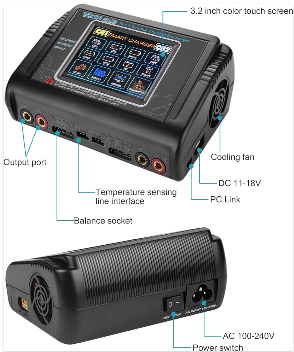
Image 4.2: Detailed view of the charger's 3.2-inch color touch screen, output ports, balance sockets, cooling fan, and power inputs.
