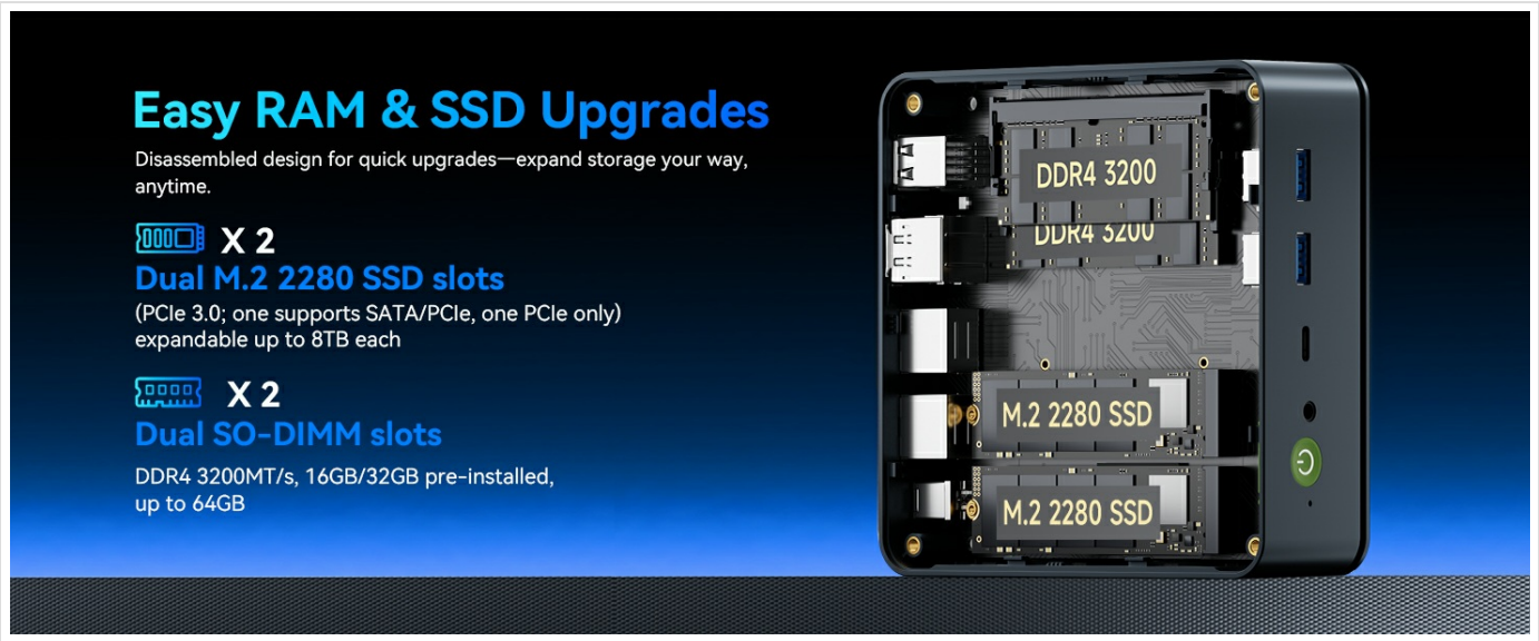
Image: An internal view of the GMKtec M5 Ultra Mini PC, illustrating the dual SO-DIMM slots for DDR4 RAM and dual M.2 2280 SSD slots for storage expansion.
