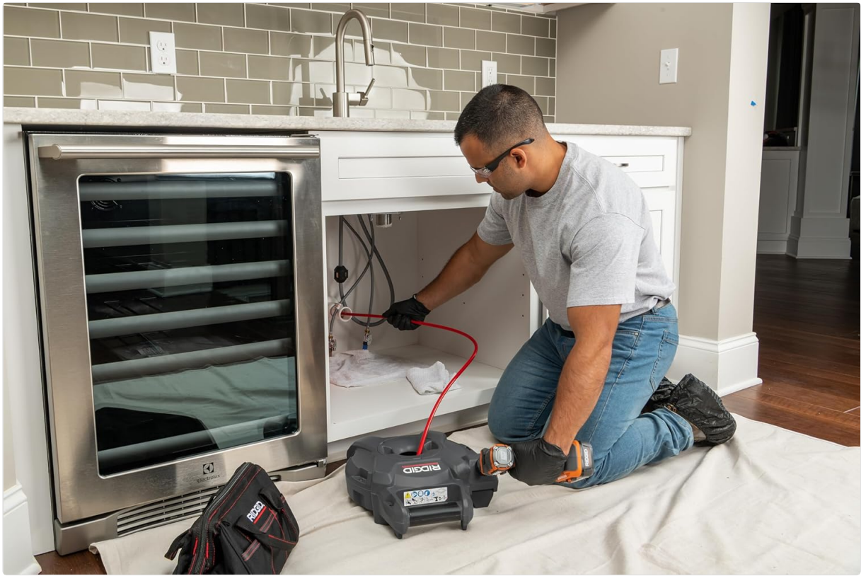
Figure 4.1: A user operating the FlexShaft K9-12 machine to clear a blockage in a kitchen sink drain.
