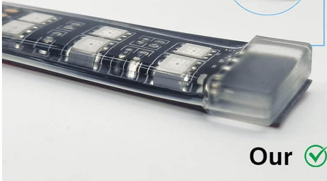
Figure 7: IP68 Waterproof design with three major protective measures.
