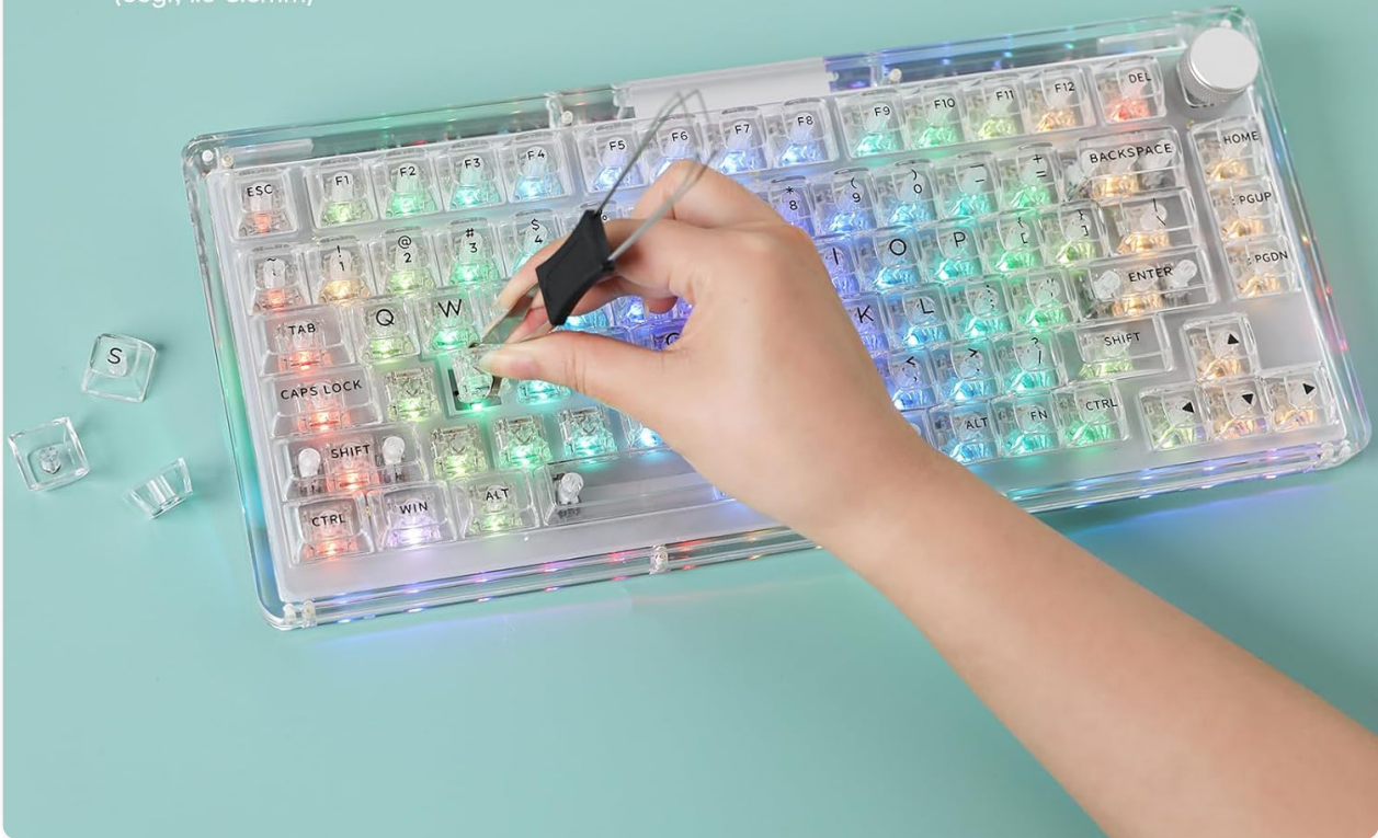
Image: A hand demonstrating the removal of a keycap and switch from the hot-swappable PCB of the KiiBoom Phantom 81 V3 keyboard.
