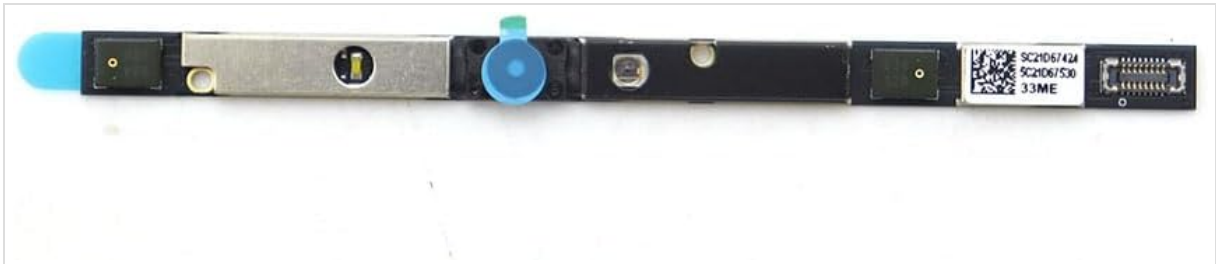
Image 1: The Generic Laptop Camera Module. This image displays the full camera module, a long, slender circuit board with the camera lens, microphone, and connector visible. The module features a blue protective cap on one end and a ribbon cable connector on the other, indicating its design for integration into a laptop's display assembly.
