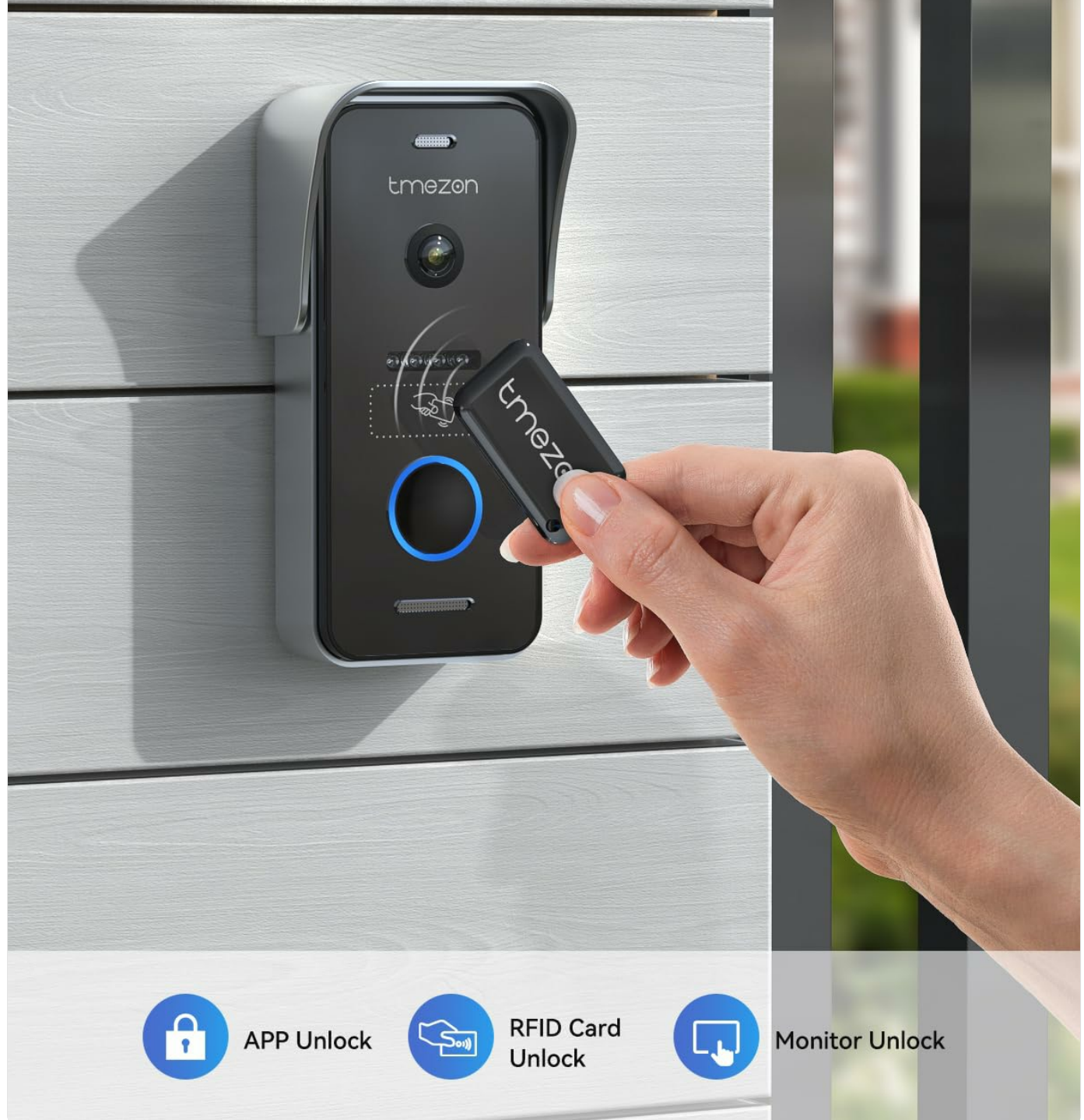
Figure 4.3: Overview of the 3-in-1 unlocking capabilities of the system.
