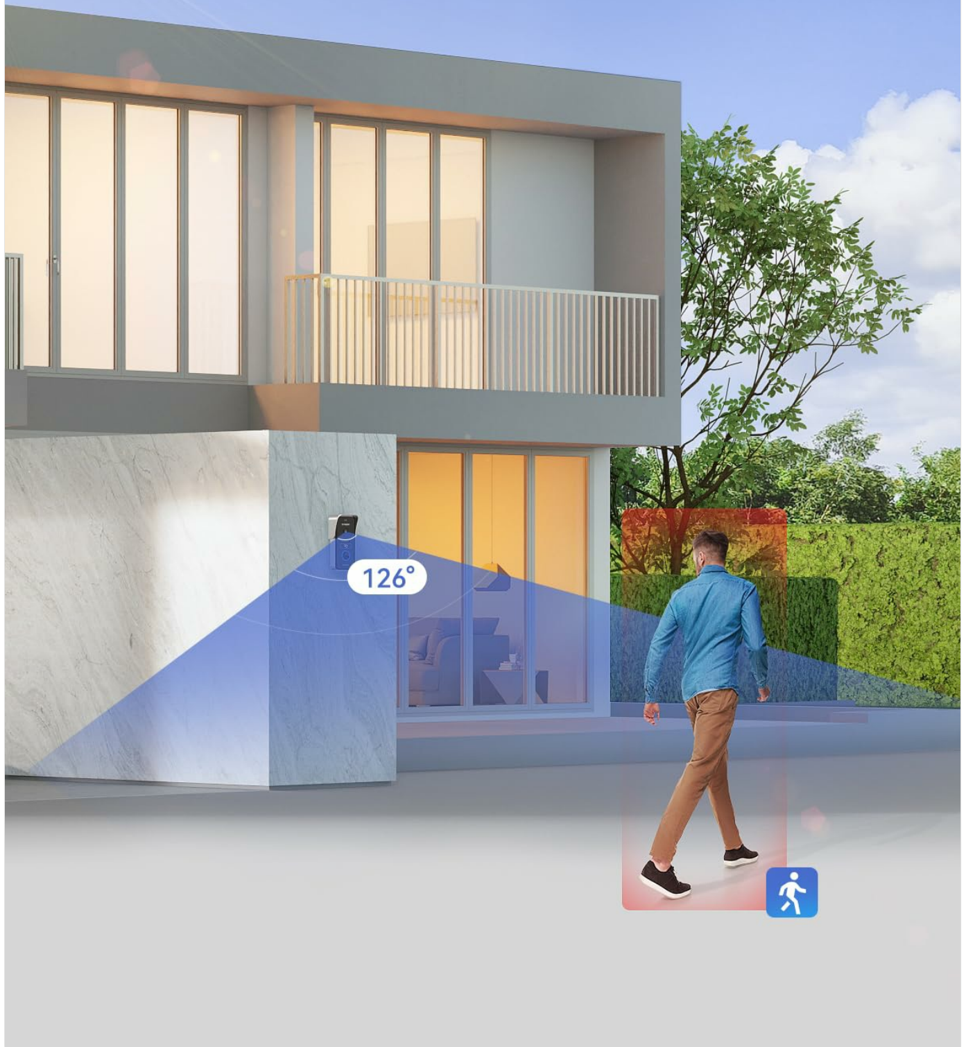
Figure 4.5: Visual representation of the smart motion detection feature and its detection range.
