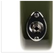
Figure 4.1: Close-up of the guitar's output jack, located on the side of the body.
