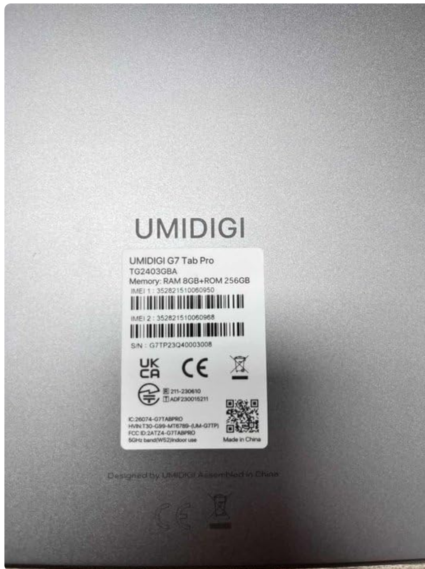
Figure 6.1: Rear view of the UMIDIGI G7 Tab Pro, displaying the model number, memory configuration, and regulatory compliance information.
