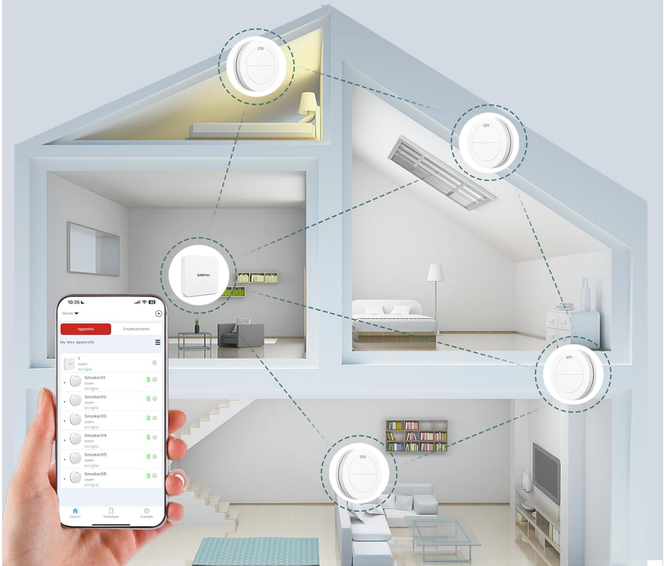
Image: An illustration showing a multi-story house with recommended locations for smoke detectors and the base station, demonstrating the interconnected network.
