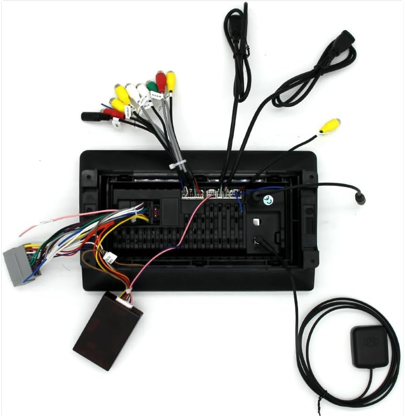
Image: The back of the car stereo unit, illustrating the various ports and wiring harnesses for power, audio, video, and peripherals.
