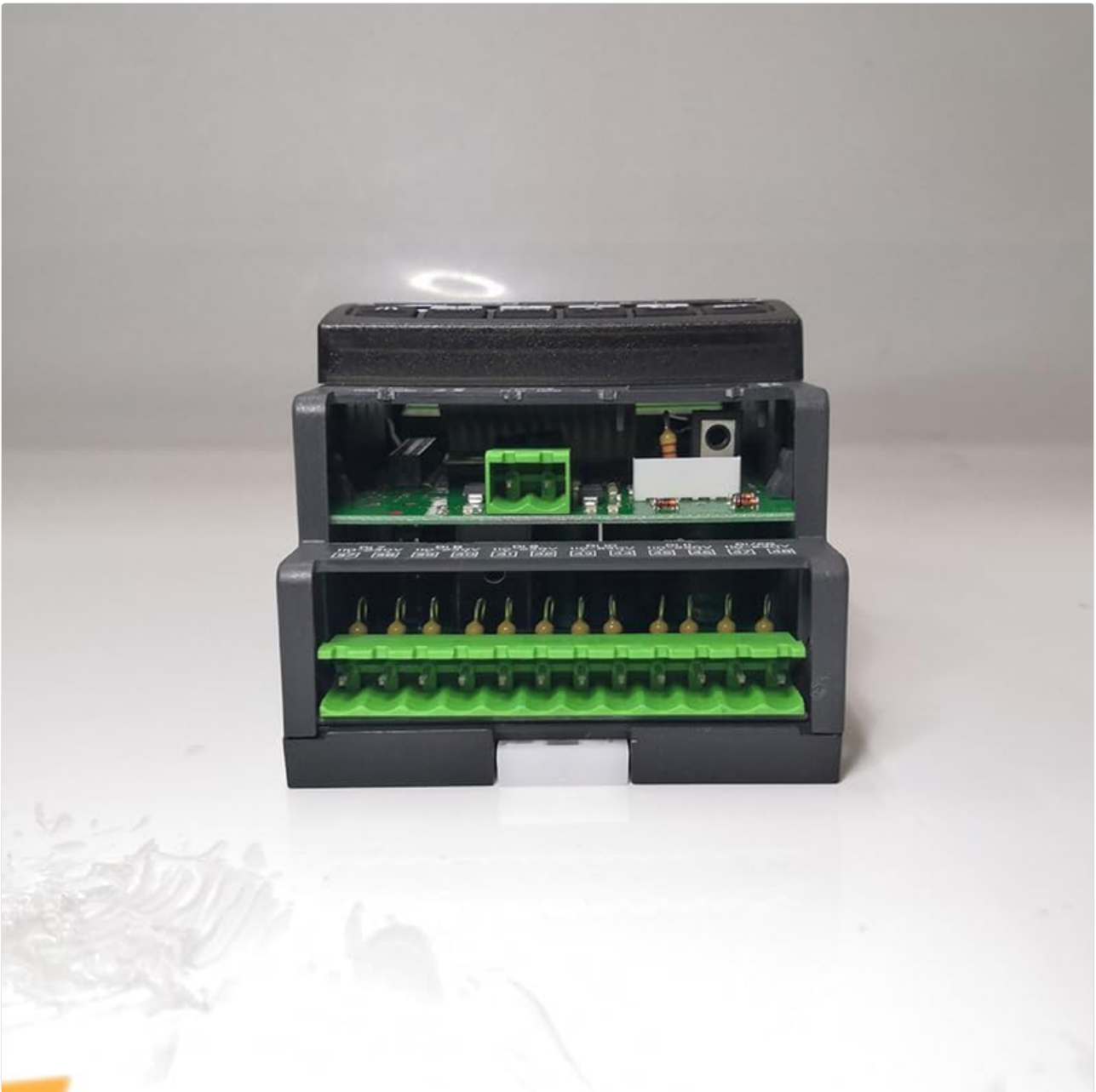
Figure 4: Bottom view of the XJM60D-21400 Controller, showing additional terminal blocks for LAN, RS485, and other connections.
