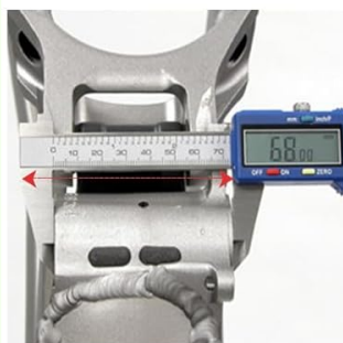
Figure 2.1: Visual guide for checking bike compatibility, including bottom bracket dimensions and chainstay clearance. It is important to measure your bike's bottom bracket inner diameter (between 33.5-36mm) and length (68-73mm). Ensure the sprocket will not interfere with your bike's chainstay.
