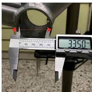
Figure 2.1: Visual guide for checking bike compatibility, including bottom bracket dimensions and chainstay clearance. It is important to measure your bike's bottom bracket inner diameter (between 33.5-36mm) and length (68-73mm). Ensure the sprocket will not interfere with your bike's chainstay.
