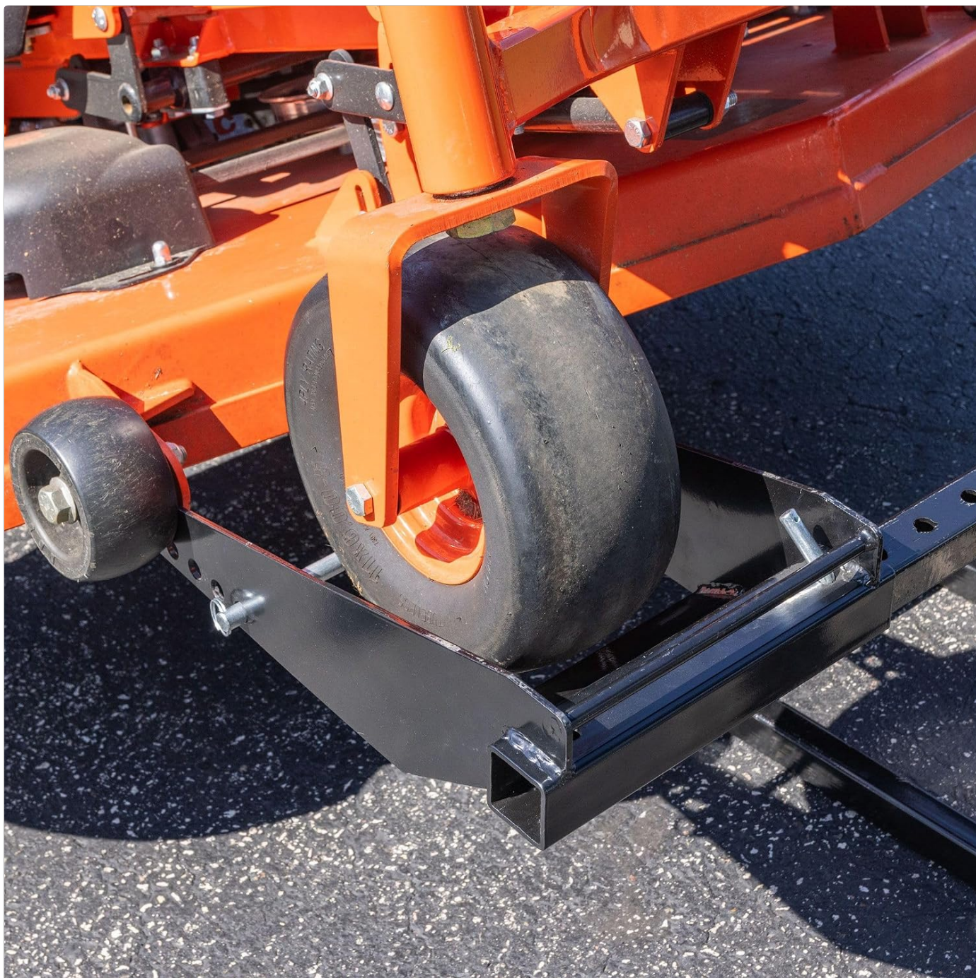
Figure 4: Mower wheel properly seated in the lift cradle.
