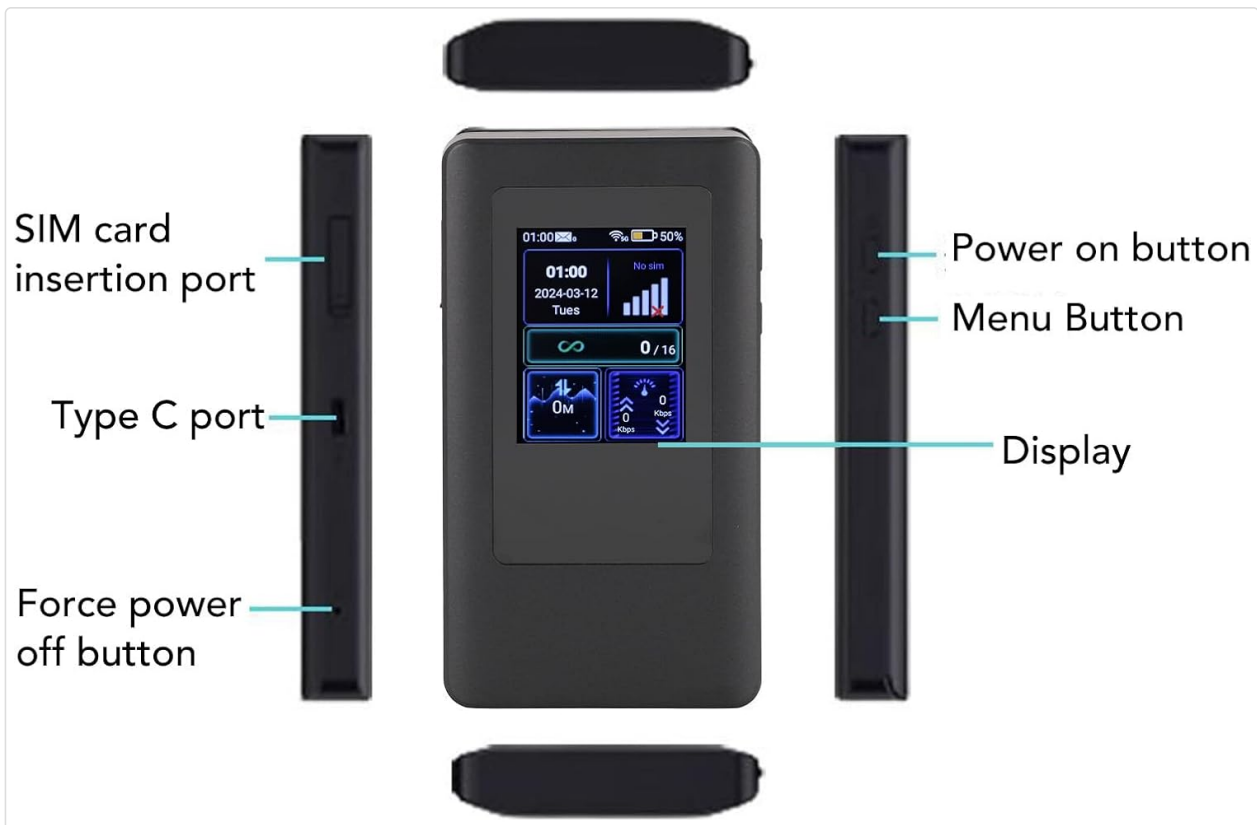
Image: A diagram illustrating the Zunate 5G Mobile Hotspot from multiple angles, highlighting key components such as the SIM card insertion port, Type-C port, Force power off button, Power on button, Menu Button, and Display.
