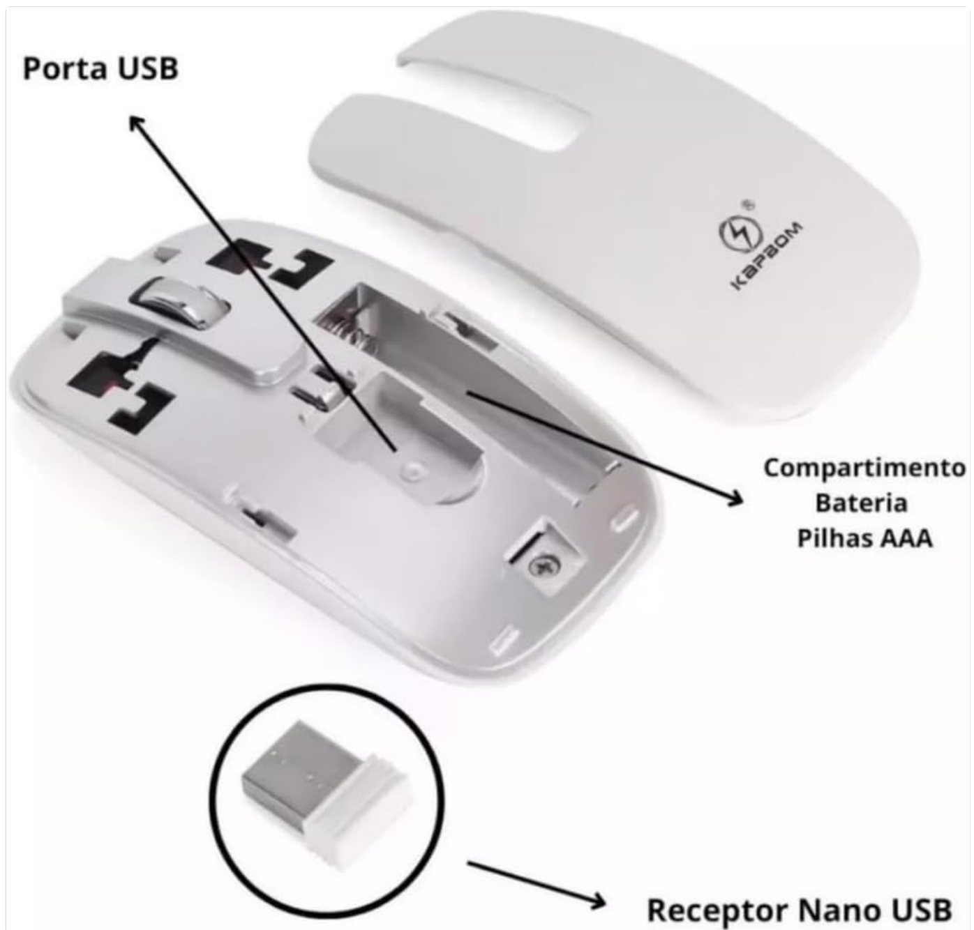
Image: Underside of the mouse showing the battery compartment and the storage slot for the Nano USB Receiver. The image points to the USB port, battery compartment for AAA batteries, and the Nano USB Receiver.
