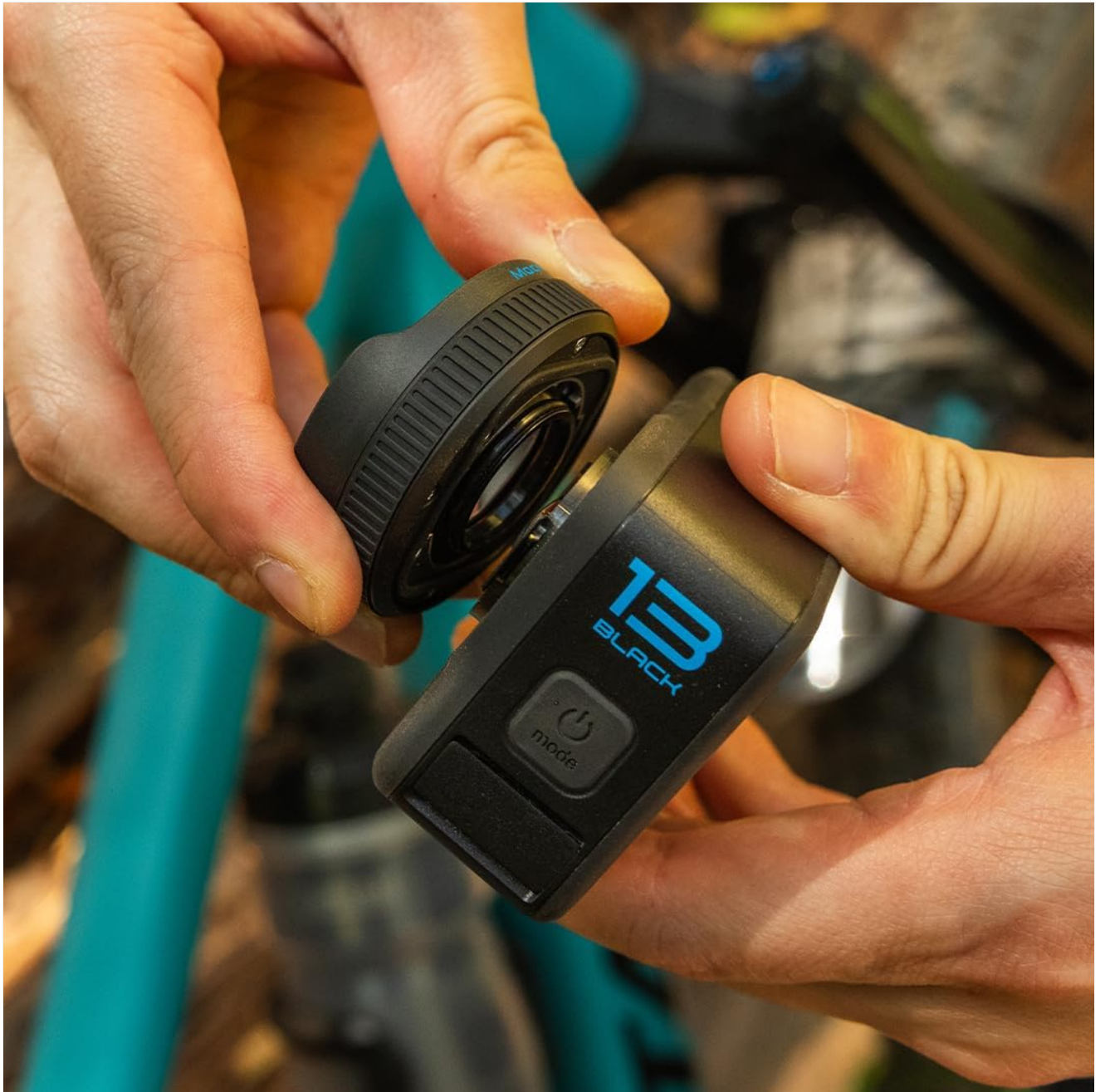
Image: Hands demonstrating the removal of the standard lens from the GoPro HERO13 Black camera.
