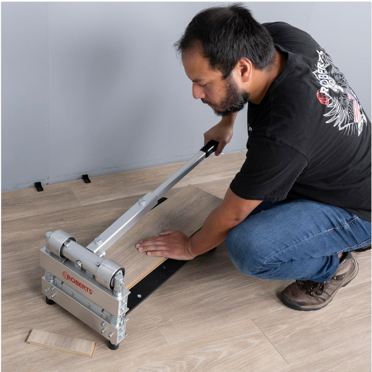
Image 5.2: User operating the cutter. This image shows a person kneeling and using the extended handle to cut a piece of flooring material, demonstrating proper technique.
