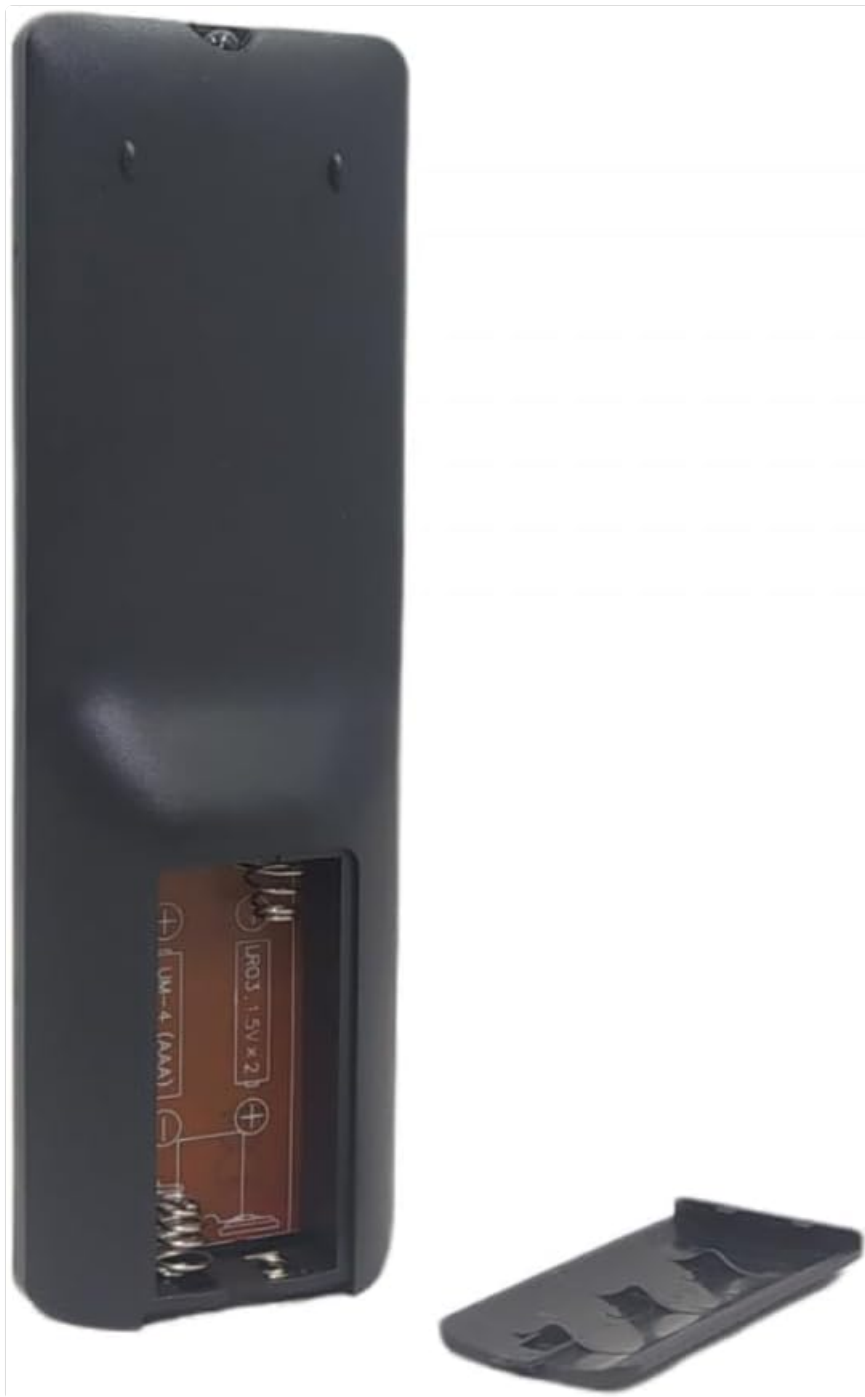
Figure 2: Battery Compartment. This image shows the back of the remote control with the battery cover removed, revealing the compartment for two AAA batteries. The positive and negative terminals are clearly marked.
