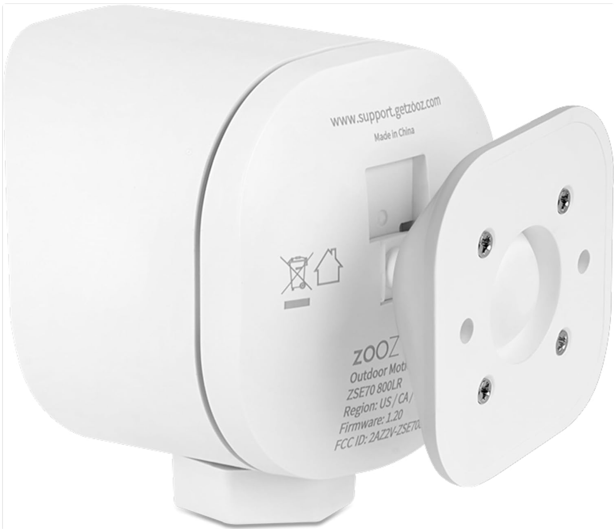
A rear view of the Zooz ZSE70 sensor, displaying its mounting plate and a label with support website and FCC ID.
