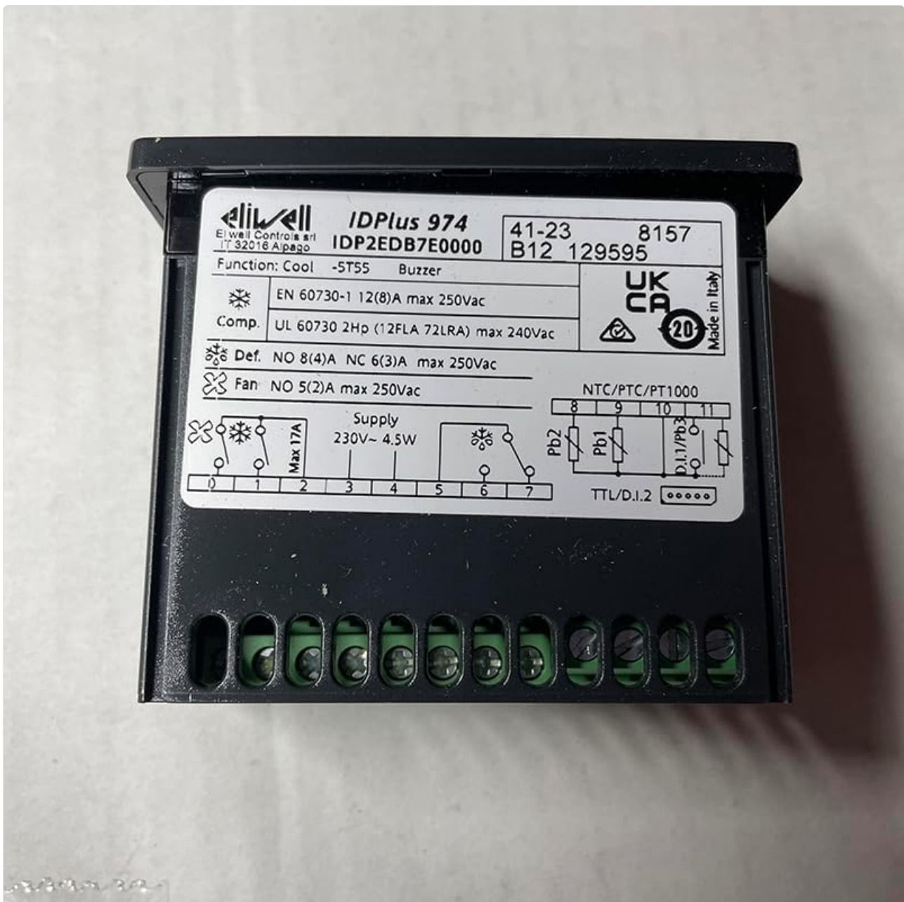
Figure 3: Top view of the IDplus 974 Temperature Controller, displaying the product label with model information, electrical ratings, and a simplified wiring schematic.
