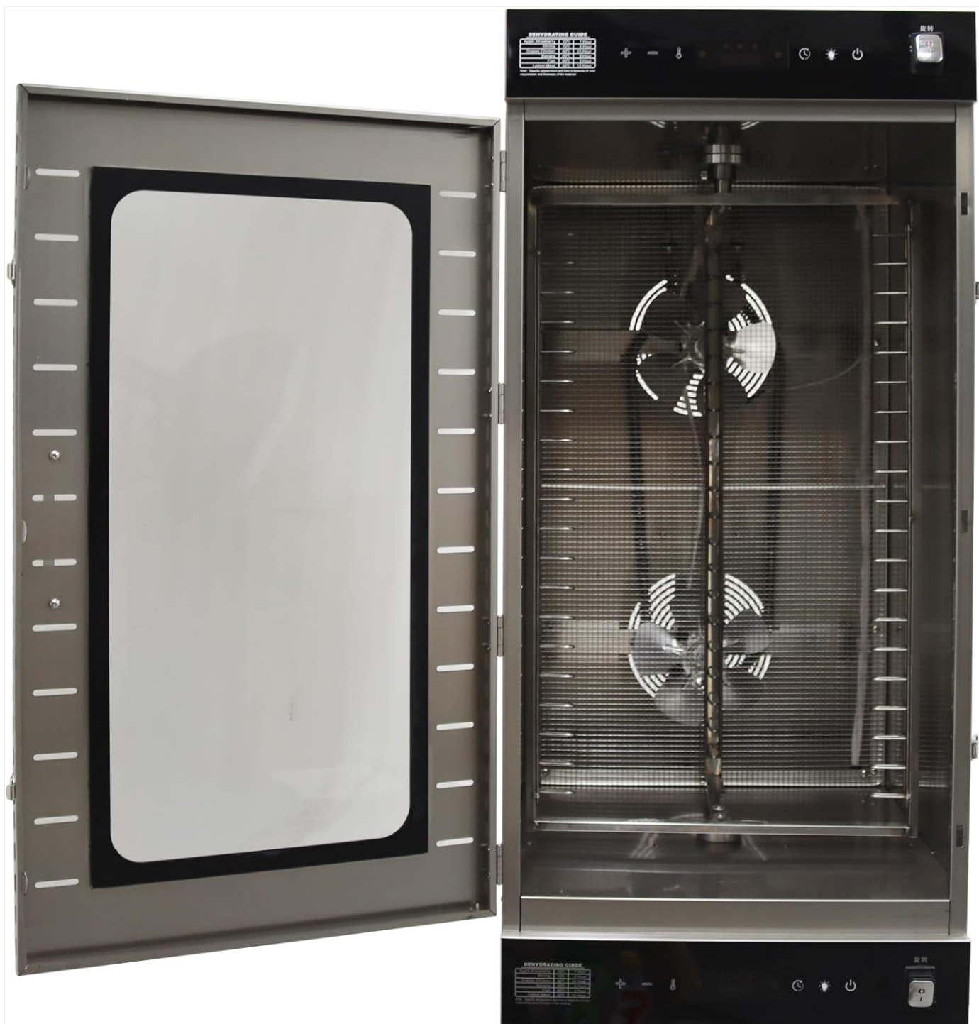
Image 7.1: Interior view of one drying chamber, showing the internal fans responsible for horizontal air circulation and even heating.
