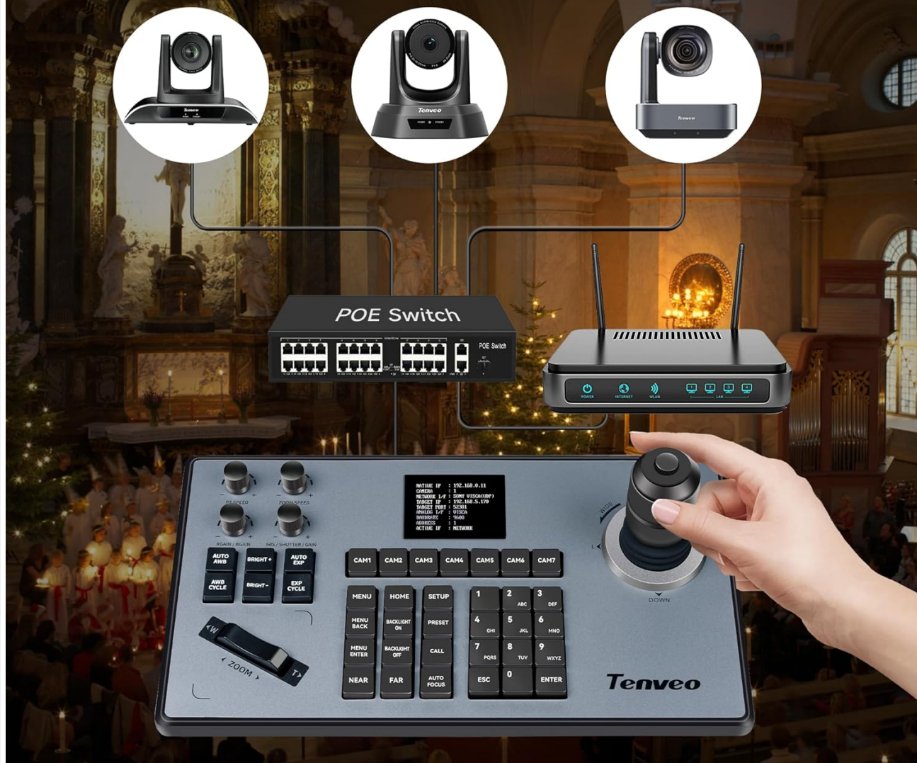
Image 5.3: Example connection diagram for multiple cameras and controller.
