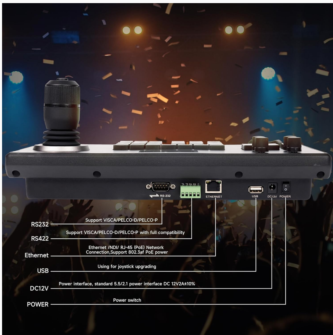
Image 5.2: KB200 Controller rear panel connections.
