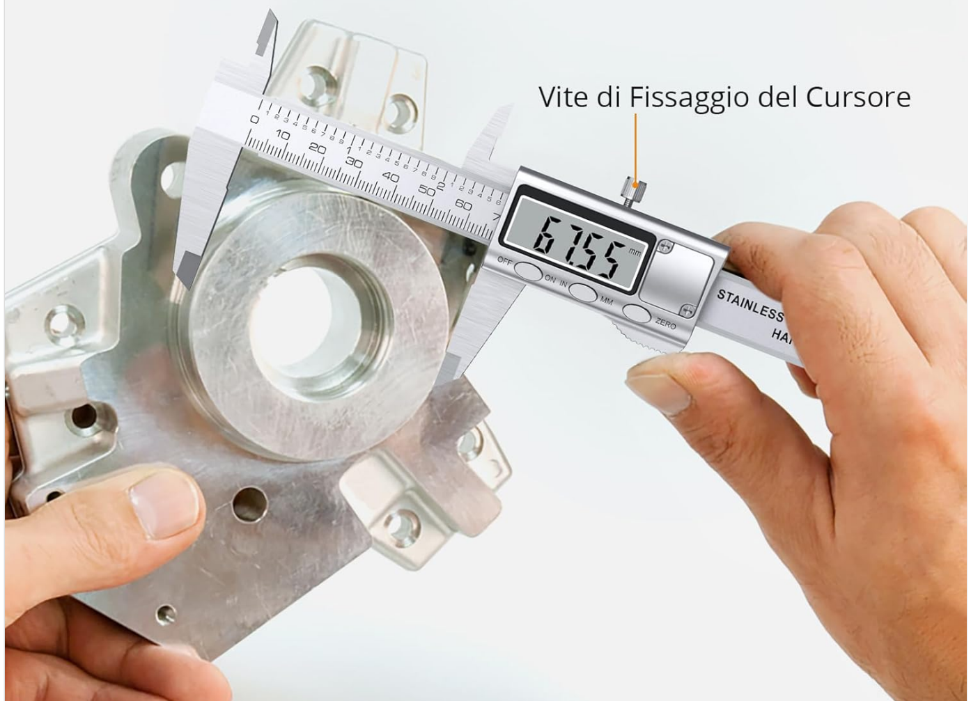
Image: The digital caliper in use, highlighting the locking screw for securing measurements.
