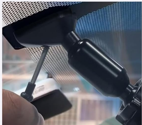
4. Tighten the screw on this bracket to fix it on the base.
