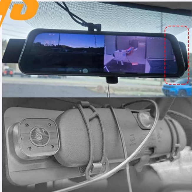
Figure 5: Comparison of OEM bracket installation versus strap mounting.
