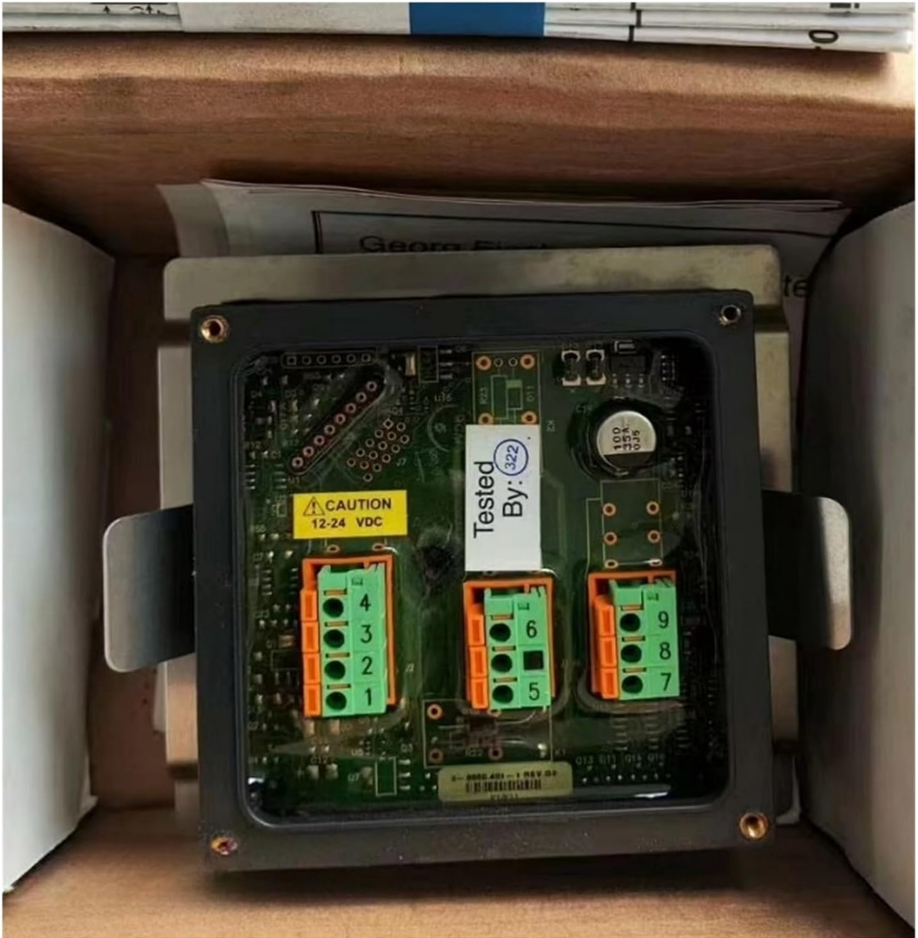
Figure 2: Internal view of the 385501P Signet Flow Conductivity Transmitter Sensor. This image displays the main circuit board with various electronic components. Prominently featured are three green terminal blocks for electrical connections, labeled with numbers (1-3, 4-6, 7-9). A yellow sticker indicates "CAUTION 12-24 VDC", specifying the required power input. Another sticker reads "Tested By: (322)", indicating quality control.
