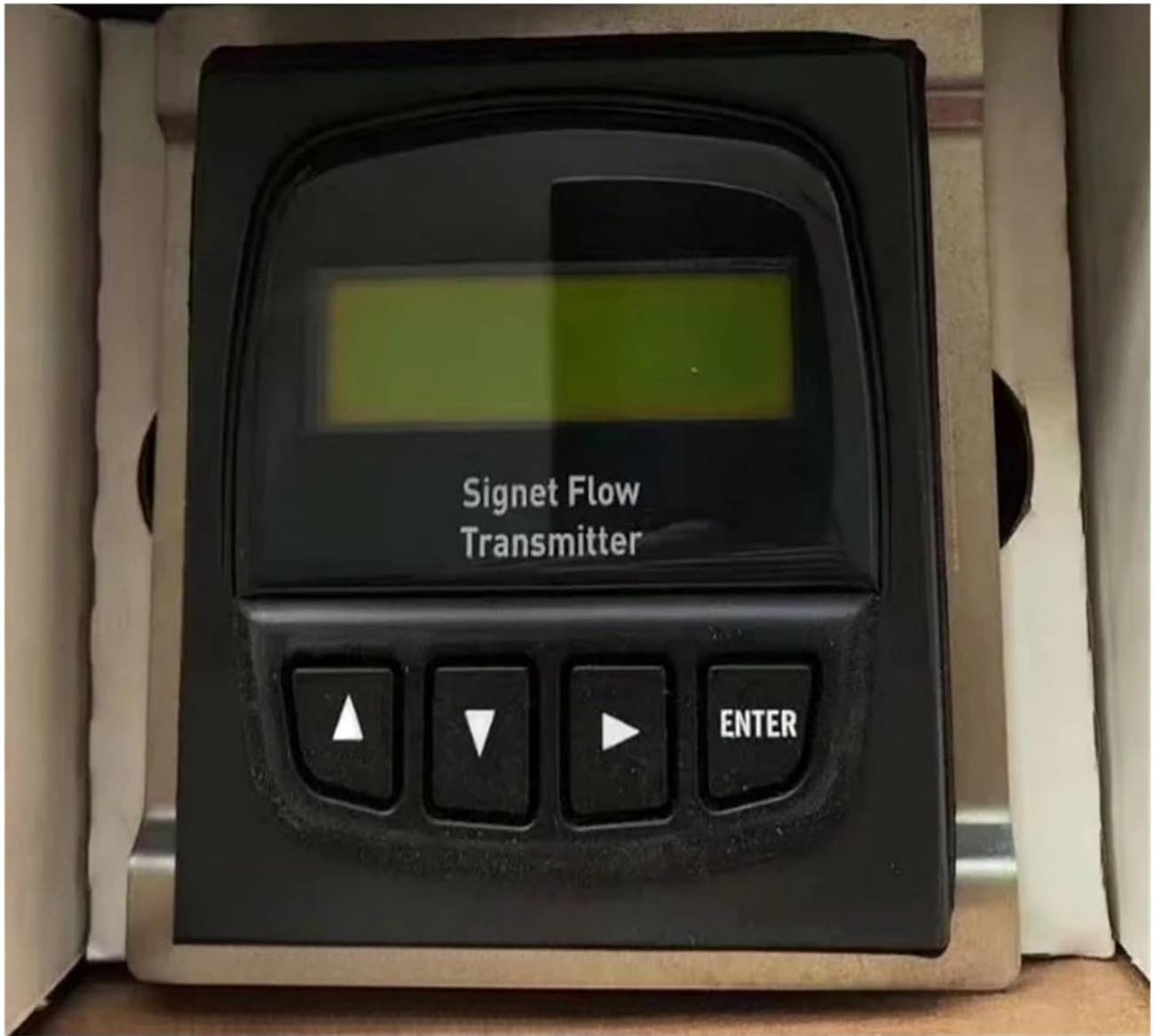
Figure 1: Front view of the 385501P Signet Flow Conductivity Transmitter Sensor. This image shows the main display screen, which typically presents conductivity readings, and the four control buttons: two arrow buttons for navigation, a right arrow button, and an 'ENTER' button for selection and confirmation. The text "Signet Flow Transmitter" is visible below the screen.
