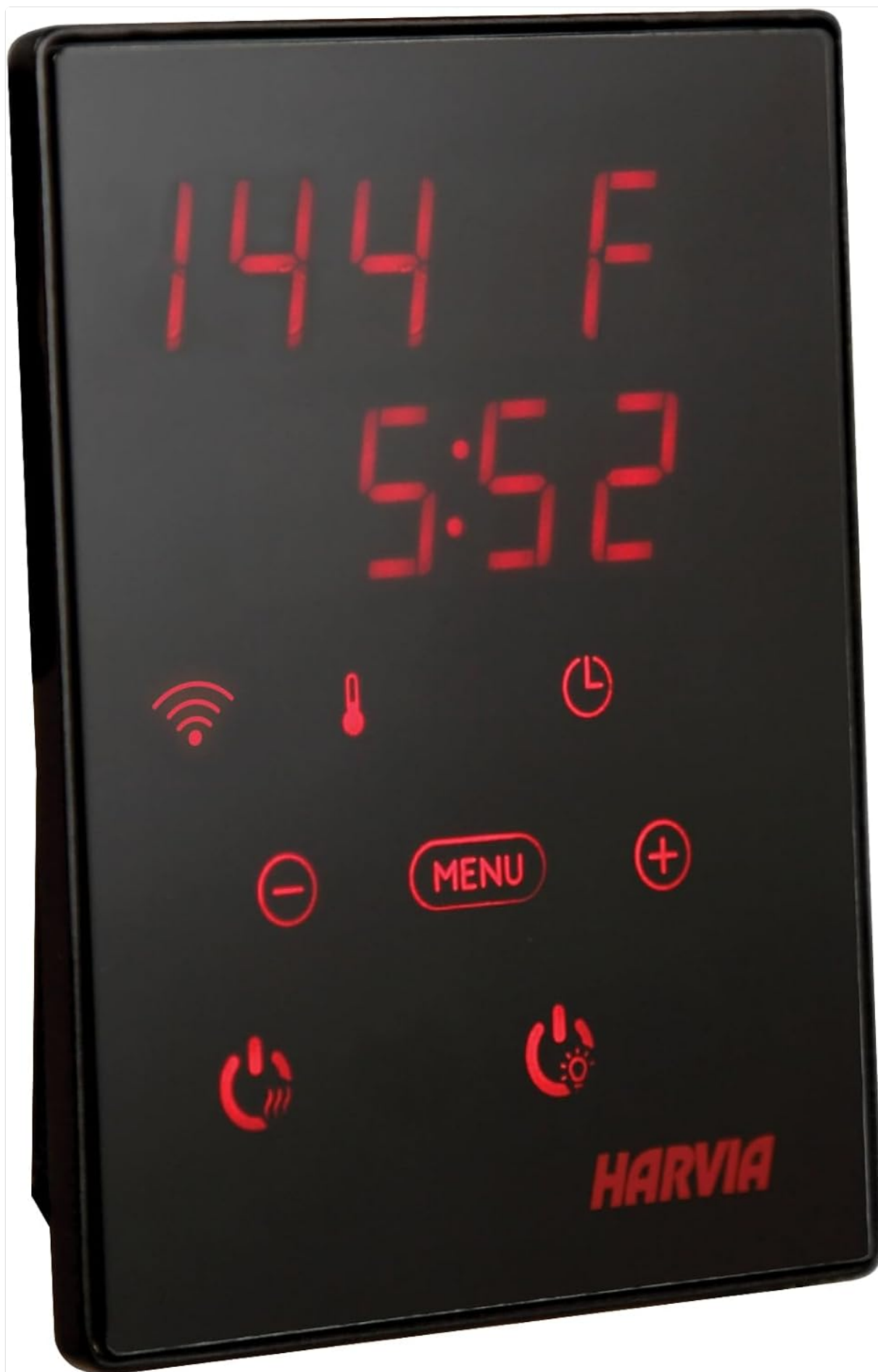
Image: The Harvia Xenio control unit display, showing temperature and time settings, along with various control icons for easy operation.
