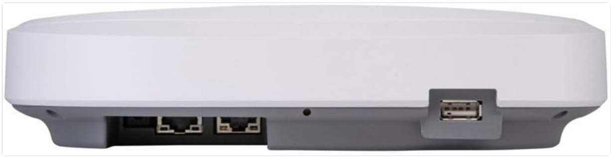
Figure 2.2: Rear view of the Ruckus R670 Access Point showing connectivity ports. This image displays the underside and rear edge of the Ruckus R670, revealing its various ports. Visible ports include two Ethernet ports and a USB port, along with a power input jack. These ports facilitate network connectivity and power supply for the device.
