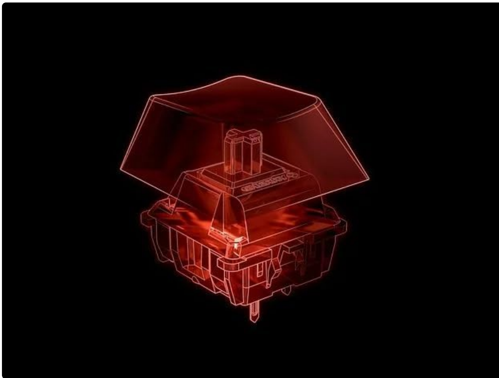
Figure 3.2: Detail of a CHERRY MX2A Switch
