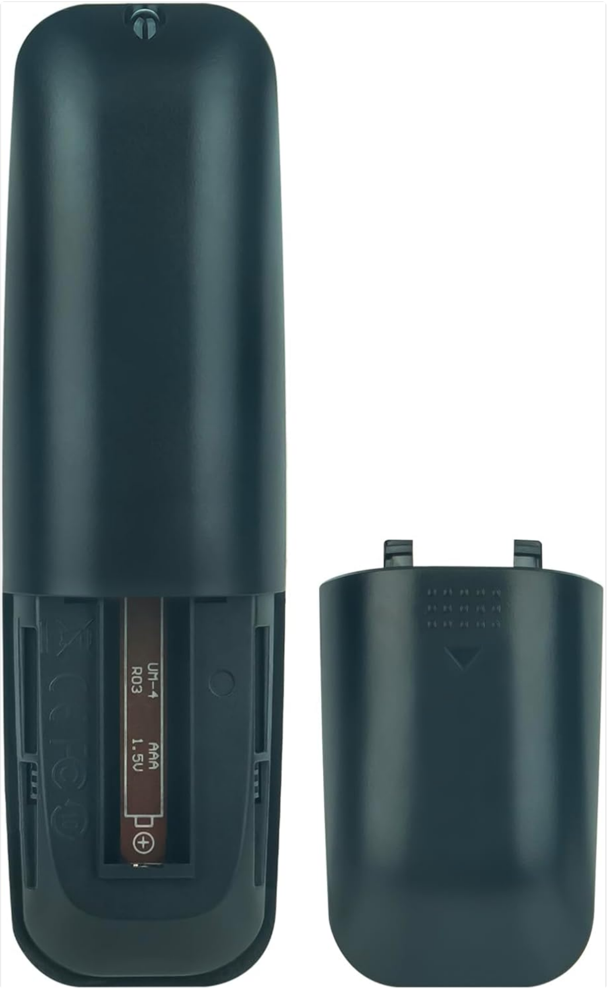
Figure 3: Rear view of the remote control with the battery cover removed, illustrating battery insertion.
