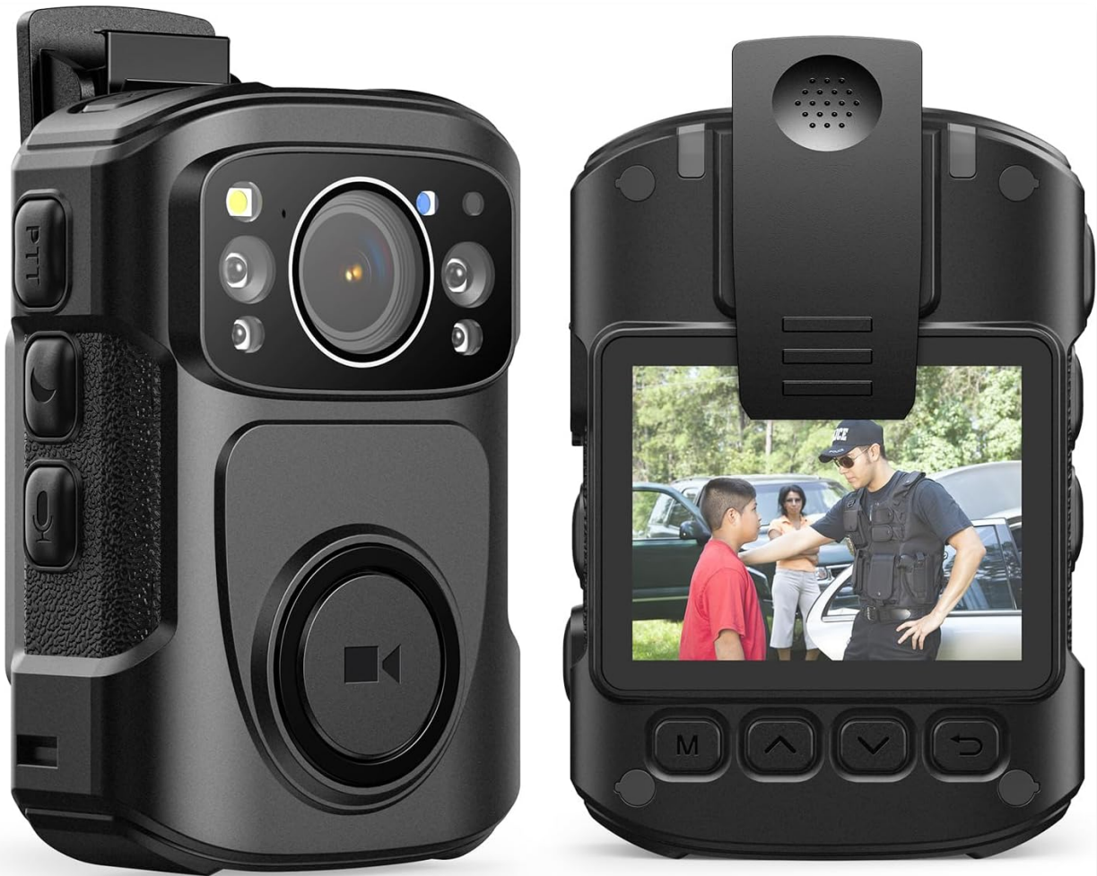
Figure 2.3: Front and back view of the BOBLOV B4K5 Body Camera, highlighting the display and navigation buttons.
