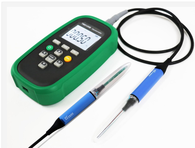
Figure 5: The TM5120B Gaussmeter shown with the axial probe connected and ready for use.
