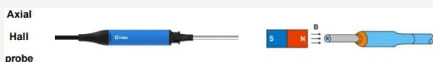
Figure 3: Diagram illustrating the axial Hall probe and its orientation relative to a magnetic field for measurement.
