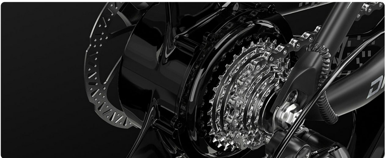
Figure 7: The 7-speed gear cassette, part of the bike's drivetrain.
