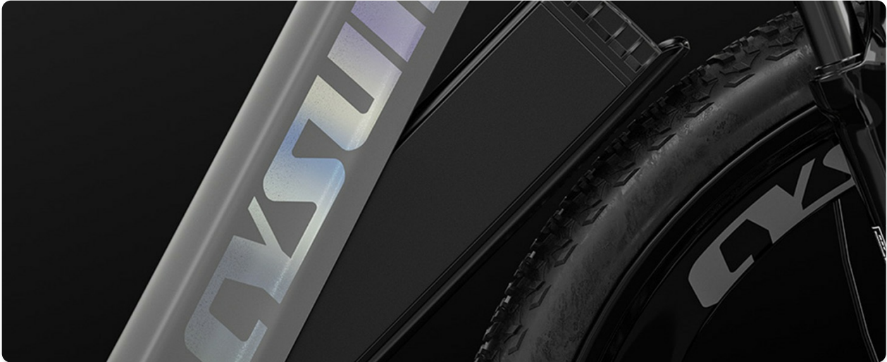
Figure 5: The integrated battery design within the e-bike frame.
