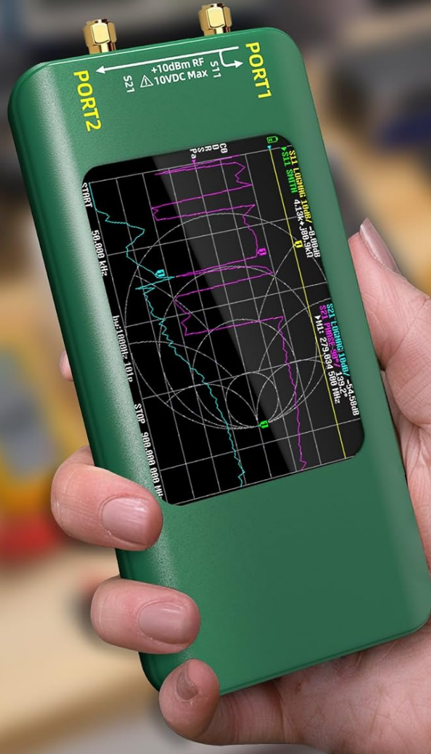
Figure 1.1: The BSIDE Vector Network Analyzer in use, highlighting its portable design, TFT color LCD, 3000mAh battery, and overall compact form factor for ham radio antenna analysis.
