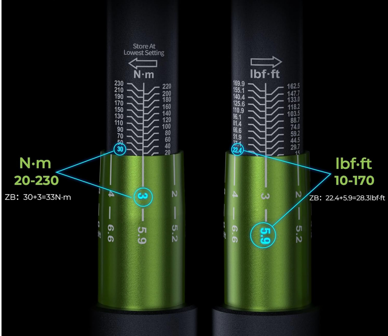
Figure 3: Detailed view of the dual-range scale, illustrating how to read both N·m (20-230) and lbf·ft (10-170) values by combining the main scale and micrometer scale readings.
