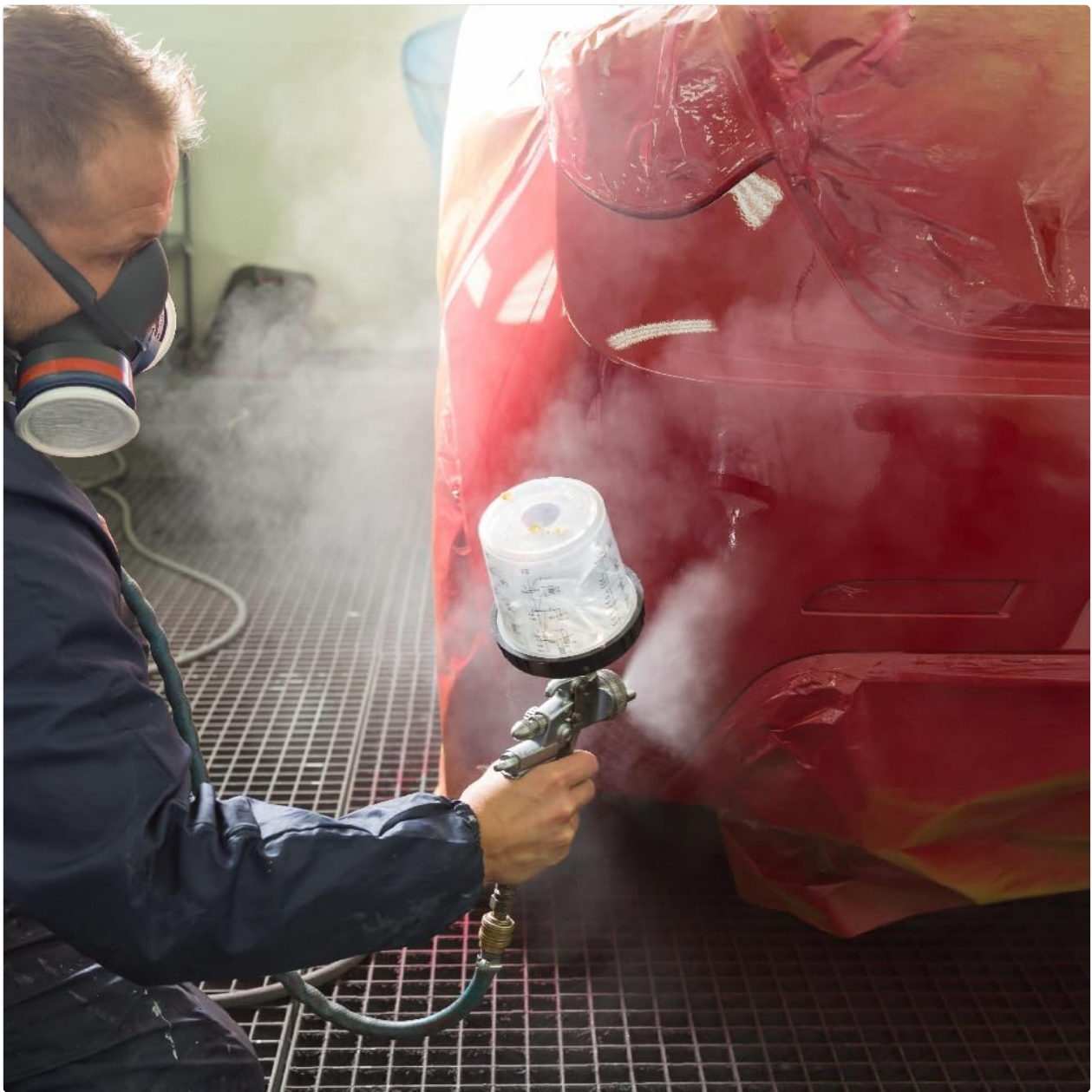
Image 4.1: An automotive technician applying clear coat in a controlled environment, demonstrating proper PPE and masking.
