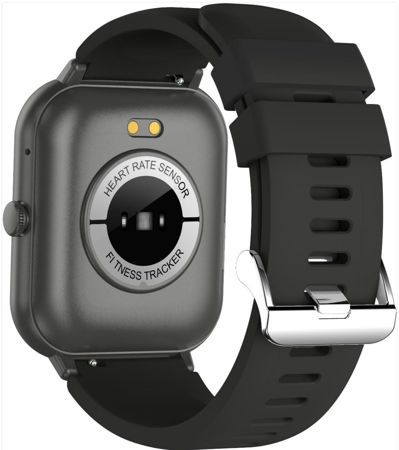
Figure 3.3: Rear view of the smart watch, highlighting the heart rate sensor and fitness tracker components.
