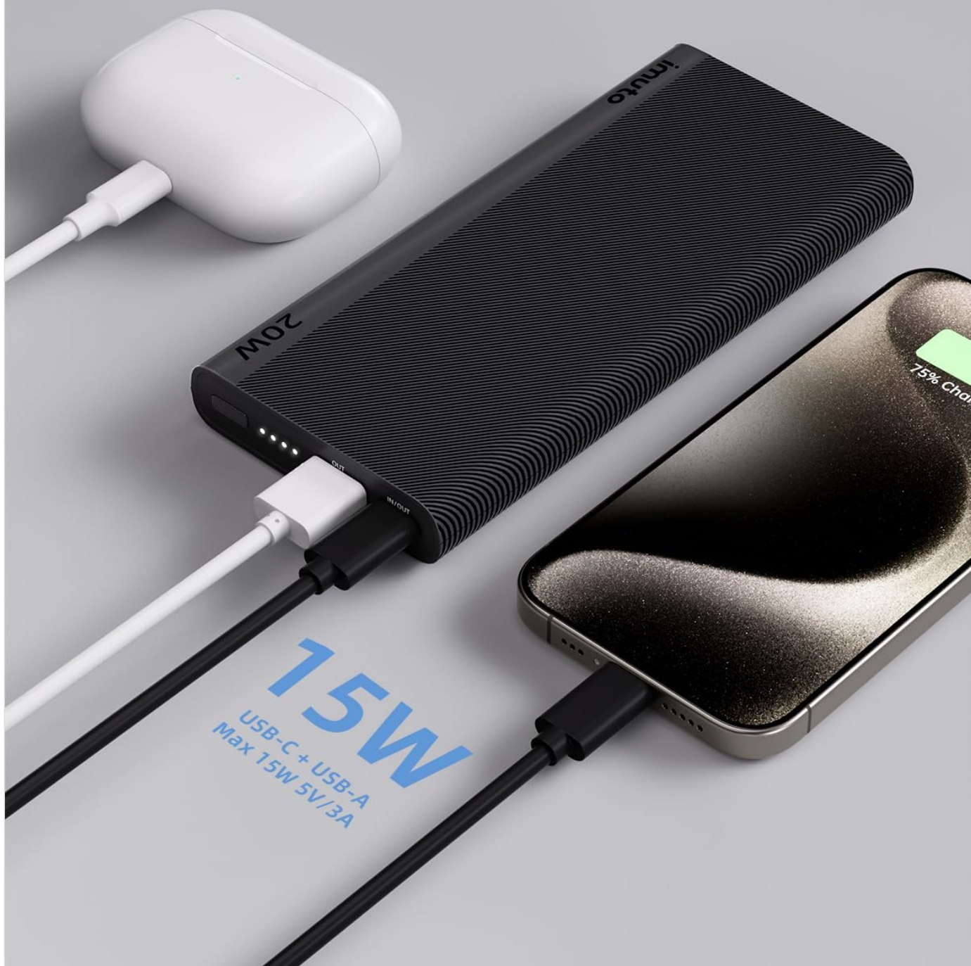
Image: The imuto portable charger is shown charging an iPhone via its USB-C port and a pair of AirPods via its USB-A port simultaneously.
