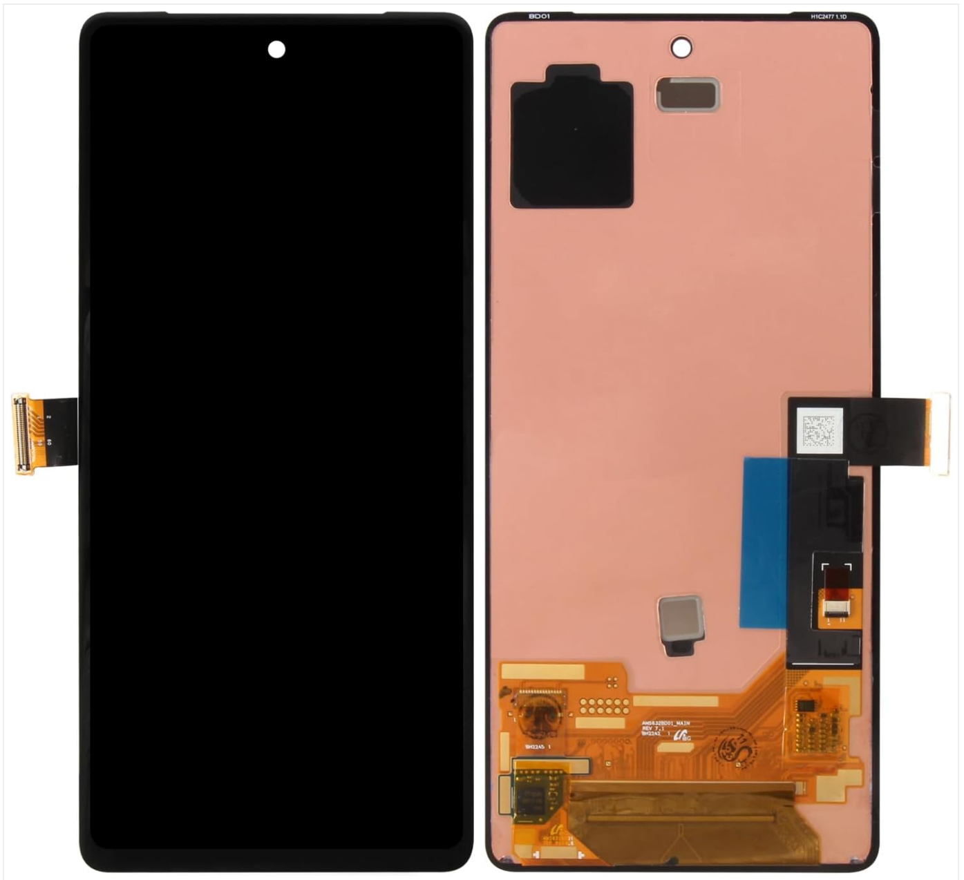
Image: A dual view of the replacement screen, showing both the front display surface and the rear side with its flex cables and connectors.
