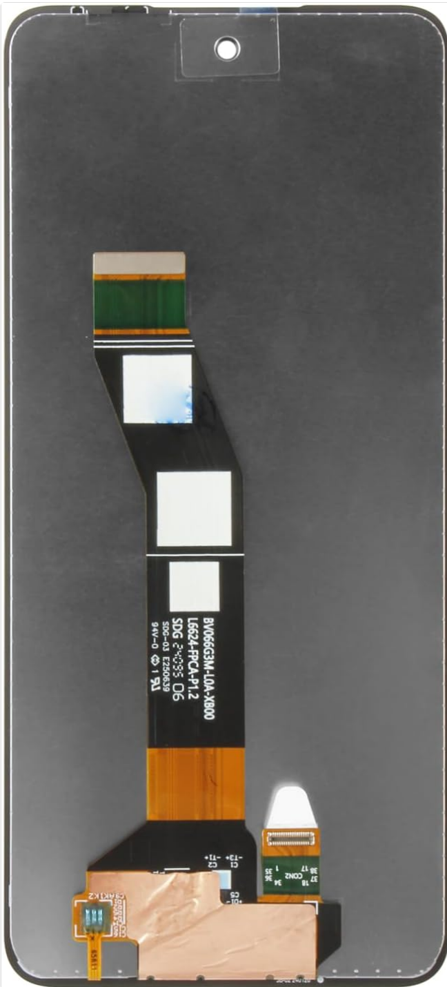
Image 4.1: The replacement screen without a frame, emphasizing the need for careful handling during installation.
