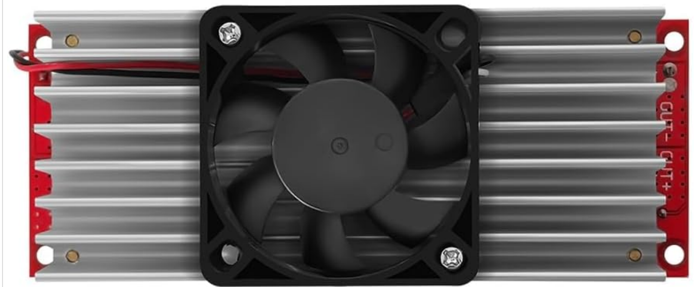
Image 2: Temperature Control Fan. This image shows the underside of the boost converter, revealing the integrated cooling fan. The fan is designed to activate automatically when the module's load temperature reaches approximately 60 degrees Celsius, ensuring optimal heat dissipation and extending product lifespan.
