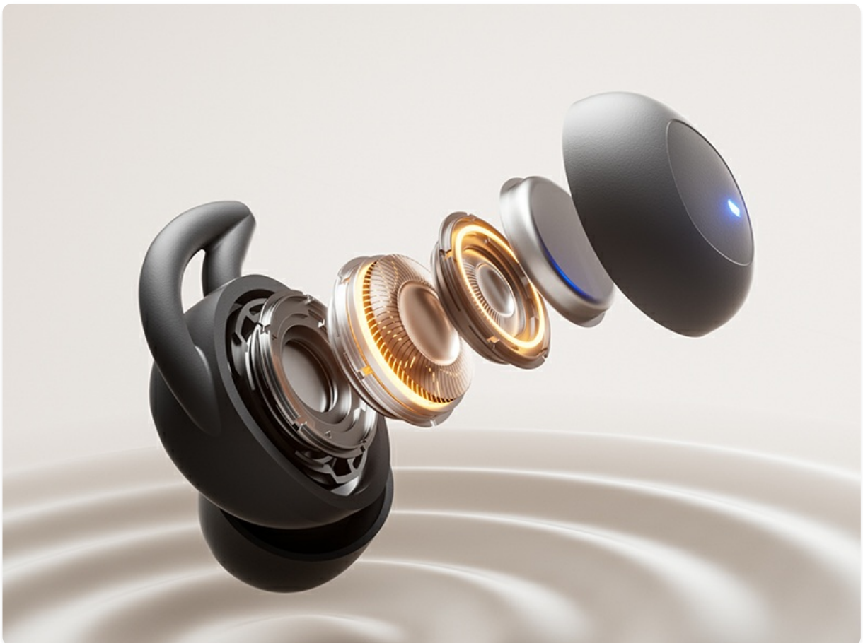
Image: Internal components of the earbud, highlighting the gold cavity speaker.
