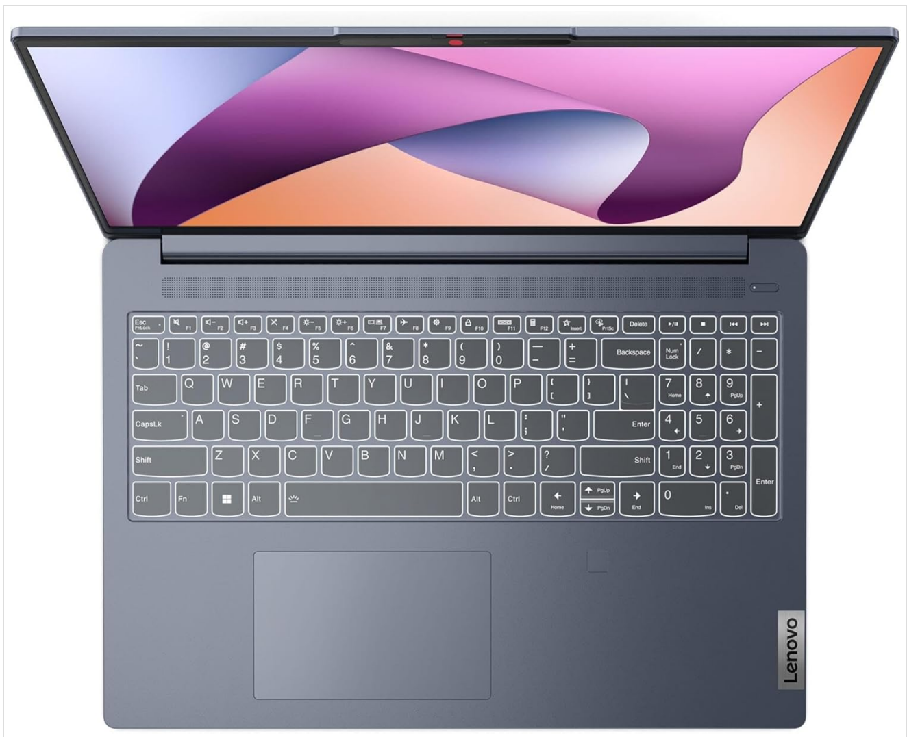
Figure 2.2.4: Top-down view of the laptop's full-size backlit keyboard with integrated Numpad and a precision touchpad.
