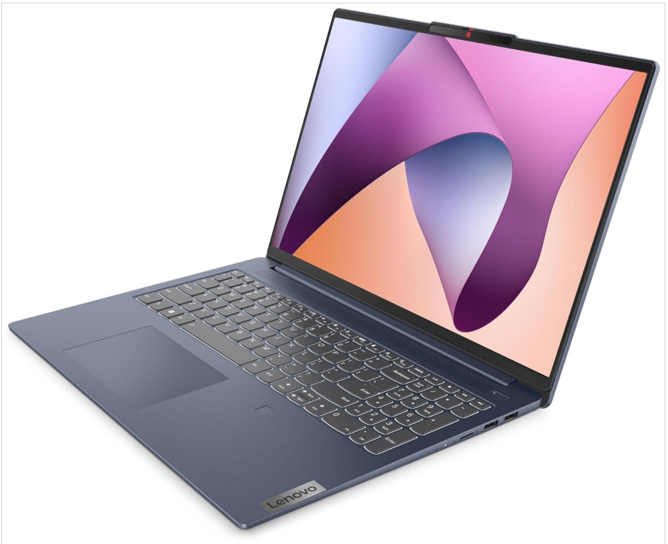
Figure 2.2.3: Right side of the laptop, equipped with two USB 3.2 Gen 1 ports and an SD card reader slot.
