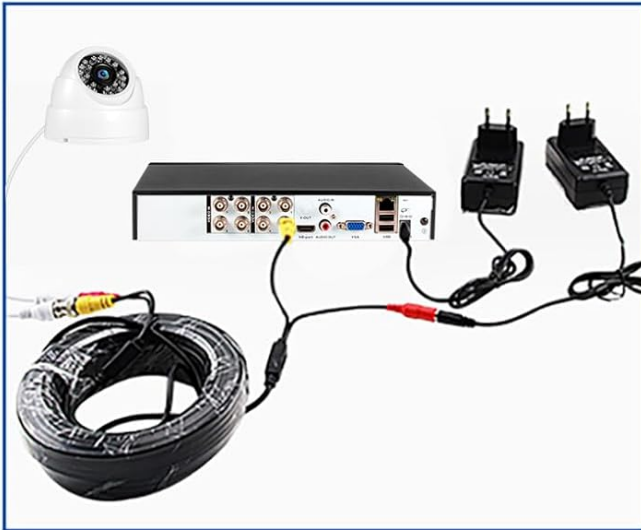
1. Connecting smart CCTV System
