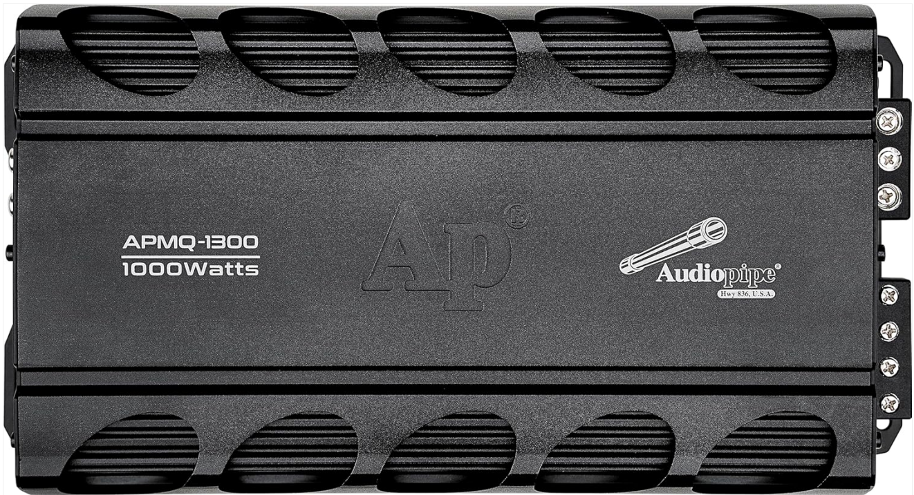
Image 5.1: Top view of the APMQ-1300 amplifier, showing the heat sink design.
