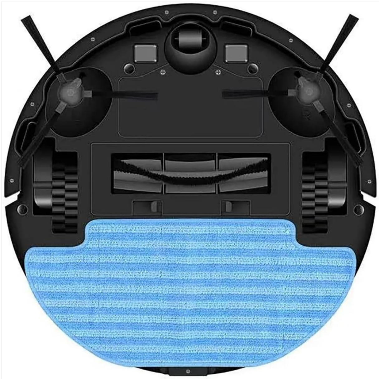
Image 2: Underside of the Liectroux ZK901 robot vacuum with the mop support and cloth installed.
